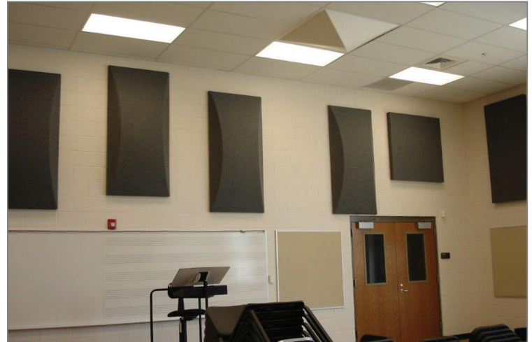
ESSI Barrel-Shaped Diffuser Panels used on walls
